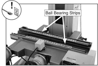
Figure 47. Table ball bearing strips exposed.
